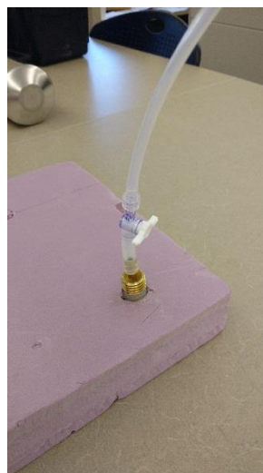
Photograph 8: Shut-In Test assembly connection to Vapor Pin®
