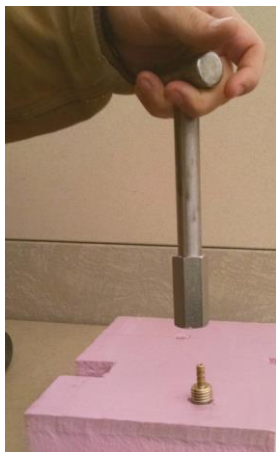
Photograph 15: Vapor Pin® Extraction
