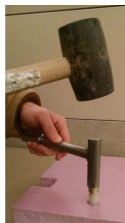
Photograph 6: Installation Tool w/ Mallet
