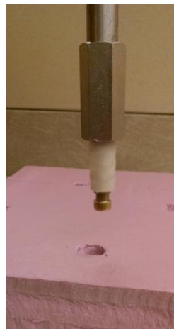
Photograph 16: Vapor Pin® Extraction
