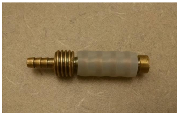
Photograph 2: Silicone tubing properly inserted onto Vapor Pin®
