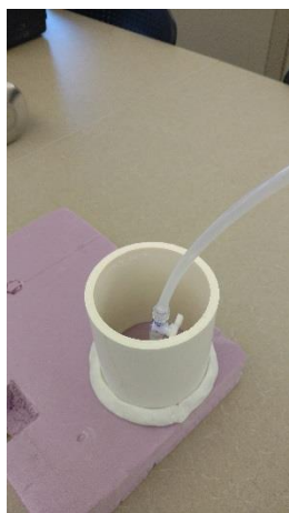
Photograph 9: Water dam around Vapor Pin®
