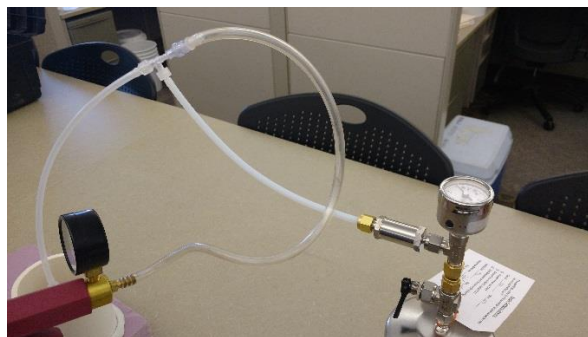
Photograph 12: Vacuum pump connected to check valve on Shut-in Test assembly
