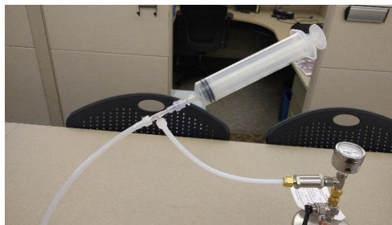
Photograph 14: Use of syringe to purge air from tubing and below ground
