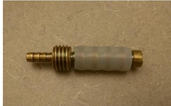
Photograph 2: Silicone tubing properly inserted onto Vapor Pin®
