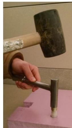
Photograph 6: Installation Tool w/ Mallet
