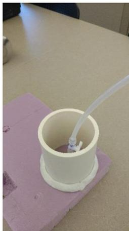
Photograph 9: Water dam around Vapor Pin®
