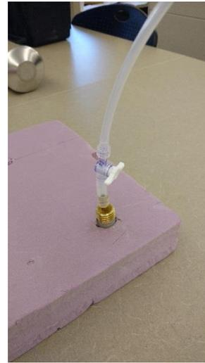
Photograph 8: Shut-In Test assembly connection to Vapor Pin®
