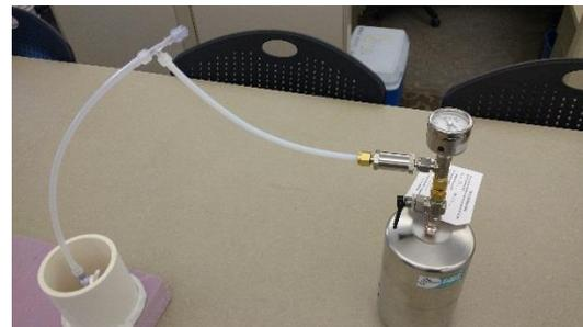
Photograph 10: Shut-In Test assembly connection to air canister
