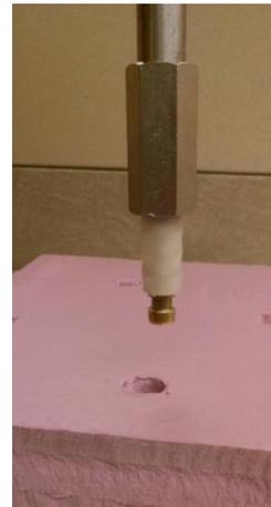
Photograph 16: Vapor Pin® Extraction
