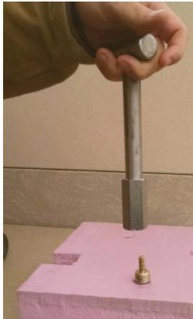
Photograph 15: Vapor Pin® Extraction
